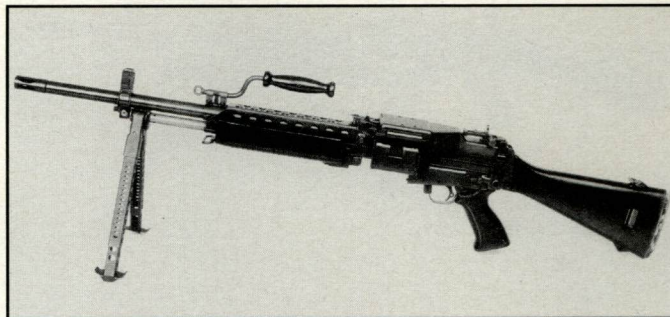
Stoner 63A light machine gun serial number 2721, left-hand belt-feed, plastic furniture, left side.
