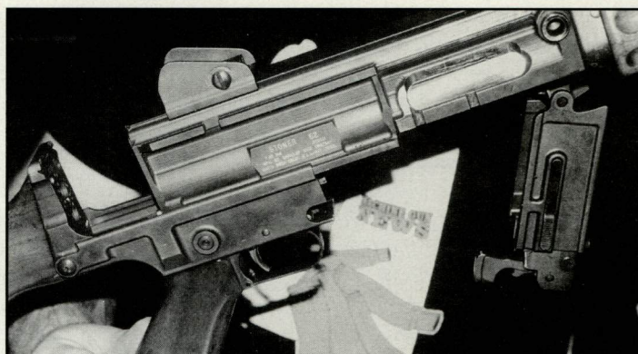
Removing Stoner 62 buttstock/trigger group. Slides to the rear.
