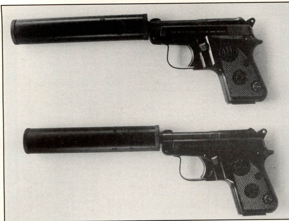
Two variants of the Beretta 950 BS pistol with Cobray suppressors: the .22 Short Minx and the .25 ACP Jetfire.
