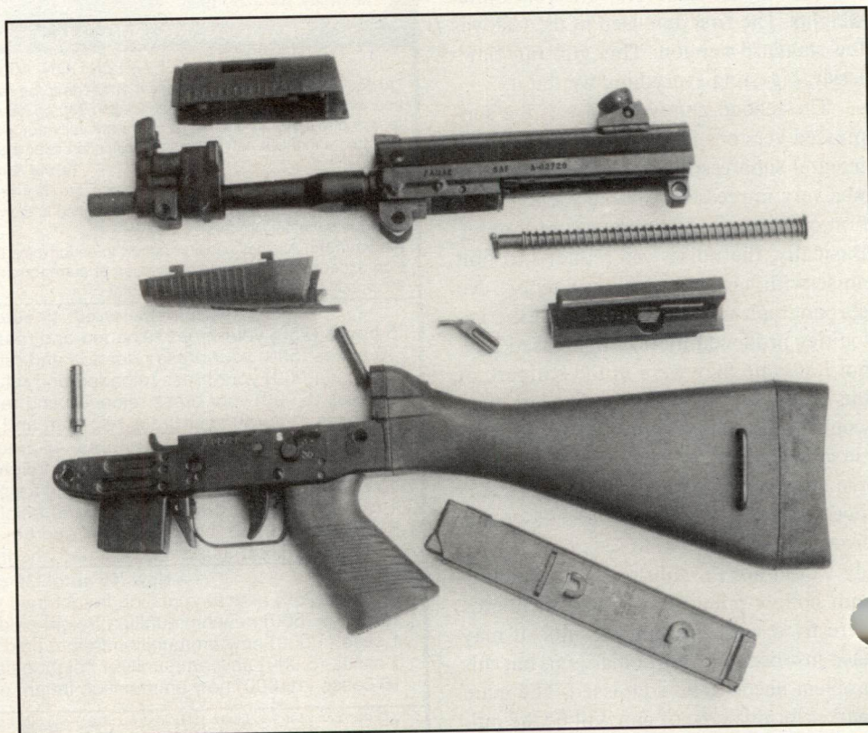
The S.A.F. takes down quickly without the need for tools. The gun is well designed and very robust. Parts will interchange between guns without problems showing good quality control.
