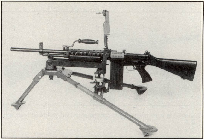
Stoner 63 serial number 234, left-hand belt-fed, heavy barrel, wooden forend, plastic furniture, 150-rd plastic box on a military M2 tripod. This has the correct cradle for the 63 which is different from the 63A top cover up.
