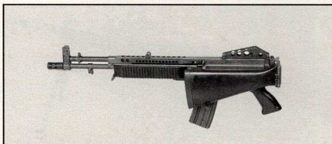
Stoner 63 carbine serial number 313, folded stock, note the new plastic forend. Left side.
